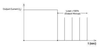
It is not recommended to prolong the duration of  $I_0$  when it is <150% but >100%, since it may cause damage to the PSU.
