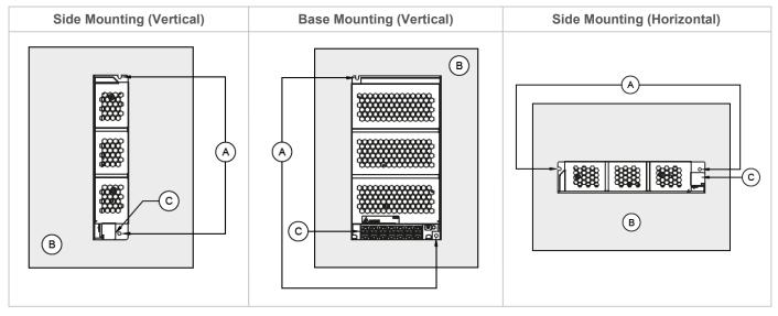
Fig. 2 Mounting Orientation
