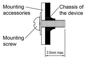
Only use M3 screw ≤ 3.5mm (0.14 inch) through the base mounting holes. This is to keep a safety distance between the screw and internal components.
