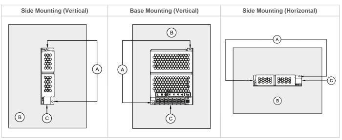
Fig. 2 Mounting Orientation
