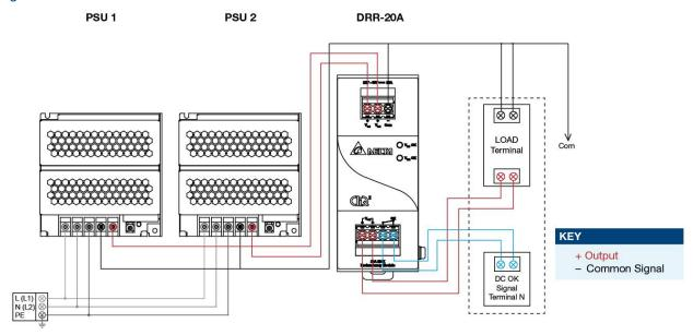
Fig. 3 Redundancy / Parallel Operation Connection Diagram
