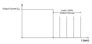
It is not recommended to prolong the duration of I<sub>O</sub> when it is <120% but >100%, since it may cause damage to the PSU.
