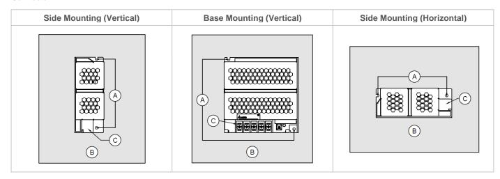
Fig. 2 Mounting Orientation
