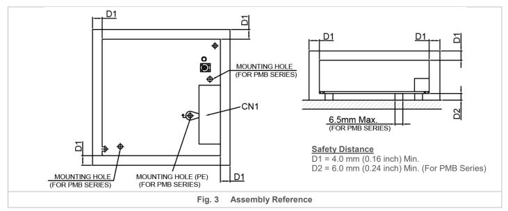
Ensure the mounted device is kept at  $\geq$  4mm (0.16 inch) safety distance at all sides from other components and equipments. In addition, to ensure sufficient convection cooling, always maintain a distance of  $\geq$  20mm (0.79 inch) from ventilated surfaces while the device is in operation.
