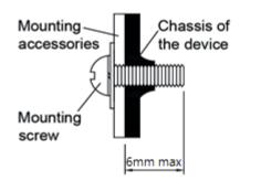
Fig. 4 Mounting Screw
