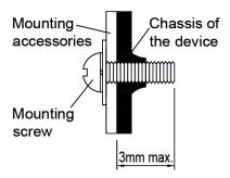
Fig. 4 Mounting Screw
