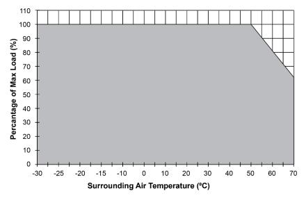
Fig. 1 De-rating for Horizontal Mounting Orientation > 50°C de-rate power by 2% / °C
