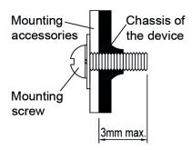
Fig. 4 Mounting Screw
