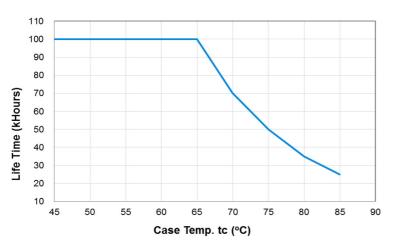
Lifetime vs. Ambient Temp. w/o Load Derating
