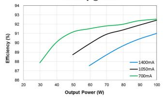
Efficiency @277Vac Efficiency (%) 1400mA 1050mA 700mA **Output Power (W)**
