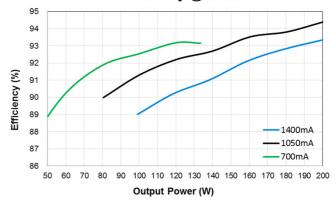
Efficiency @277Vac 95 94 93 92 Efficiency (%) 91 90 89 700mA 88 1400mA 87 -1050mA 86 50 60 70 80 90 100 110 120 130 140 150 160 170 180 190 200 **Output Power (W)**
