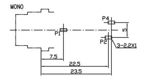
RECOMMEND PCB LAYOUT (JACK TOP VIEW) TOLERANCE: ±0.05mm RECOMMEND PCB THICKNESS: 1.6mm
