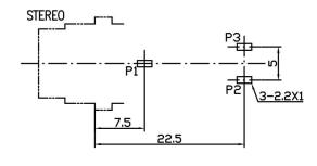
RECOMMEND PCB LAYOUT (JACK TOP VIEW) TOLERANCE: ±0.05mm RECOMMEND PCB THICKNESS: 1.6mm
