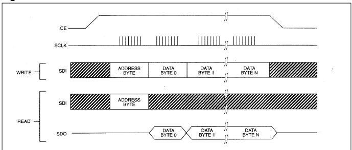
Figure 8. SPI MULTIPLE-BYTE BURST TRANSFER
