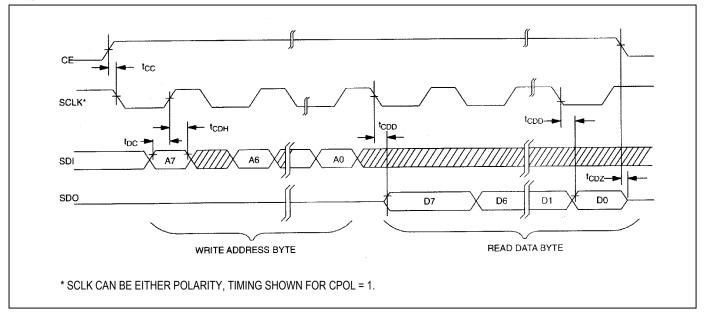
Figure 13. TIMING DIAGRAM: SPI WRITE DATA TRANSFER
