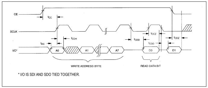
Figure 11. TIMING DIAGRAM: 3-WIRE WRITE DATA TRANSFER
