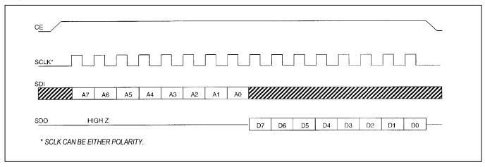
The address byte is always the first byte entered after CE is driven high. The most significant bit (A7) of this byte determines if a read or write takes place. If A7 is 0, one or more read cycles occur. If A7 is 1, one or more write cycles occur.
