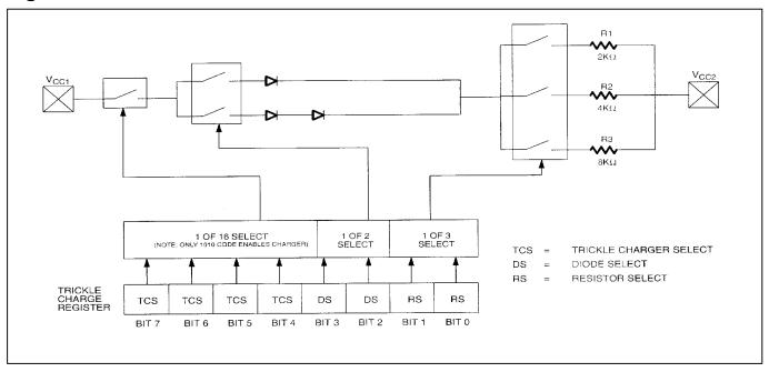
Table 2. TRICKLE CHARGER RESISTOR AND DIODE SELECT
