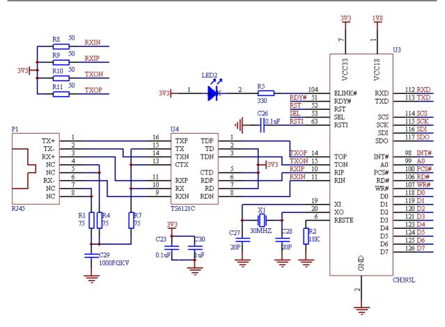
Note: for space limitation, the figure above is a schematic diagram, omitting power supply related decoupling capacitor circuit, etc. In order to improve the stability of the chip, each power pin is connected with a 0,1uF decoupling capacitor near to the ground. For detailed schematic diagram, please refer to our schematic diagram document CH395SCH.PDF.
