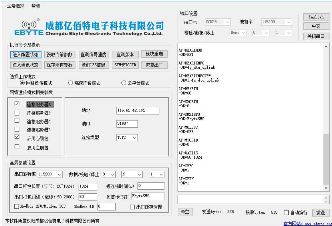
4. Query the signal strength, set the device connection server IP and port number to be: 116.62.42.192, 8124; (Ebyte test server), and finally click "Save all parameters", and finally as shown below:
