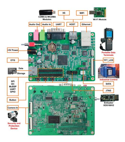
Note: Two camera interfaces and Nand Flash are on rear of the SBC8018 board
