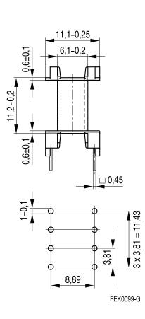
Hole arrangement View in mounting direction
