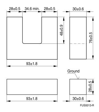
The A<sub>L</sub> value in the table applies to a core set comprising two ungapped cores.
