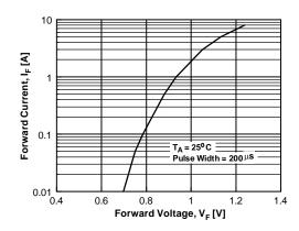
Figure 2. Forward Current Derating Curve
