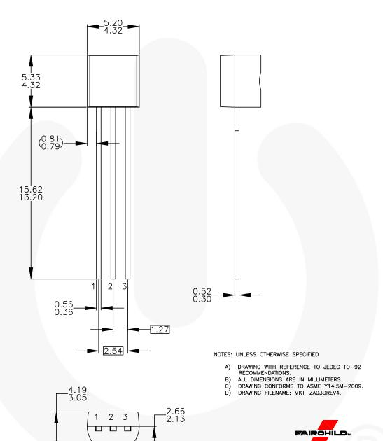
Figure 5. 3-Lead, TO-92, JEDEC TO-92 Compliant Straight Lead Configuration, Bulk Type
