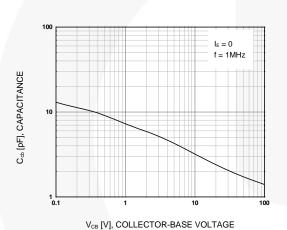
Figure 3. Collector-Base Capacitance
