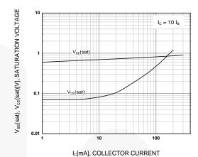
Figure 2. Collector-Emitter Saturation Voltage and Base-Emitter Saturation Voltage
