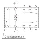
PC board mounting pad layout (TOP VIEW)
