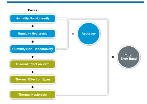
Total Error Band should not be confused with "accuracy", which is actually a component of Total Error Band. Many competitors simply specify the accuracy of their device; however, the specification may exclude hysteresis and temperature effects, and may be calculated over a very narrow range, at only one point in the range, or at their absolute best accuracy level. It is then up to the customer to calibrate the device to make sure it has the accuracy needed for the life of the application.
