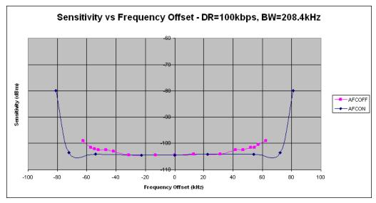
Figure 8. Sensitivity at 1% PER vs. Carrier Frequency Offset
