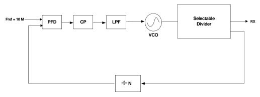
Figure 9. PLL Synthesizer Block Diagram
