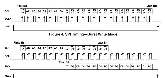
Figure 5. SPI Timing—Burst Read Mode
