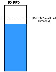
Figure 10. FIFO Threshold
