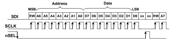
Figure 2. SPI Timing
