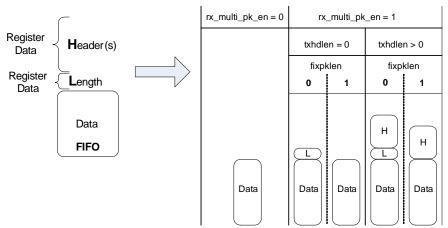
Figure 13. Multiple Packets in RX Packet Handler
