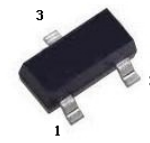
SOT-23 1. REFERENCE 2. CATHODE 3. ANODE
