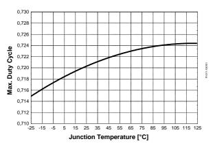
Figure 36 Max. Duty Cycle vs. T<sub>i</sub>
