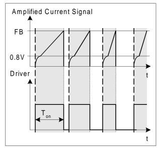
Figure 5 Pulse Width Modulation
