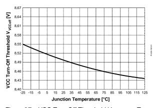
Figure 27 VCC Turn-Off Threshold  $V_{VCCoff}$  vs.  $T_i$
