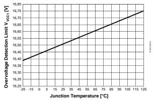
Figure 43 Overvoltage Detection Limit  $V_{VCC1}$  vs.  $T_i$
