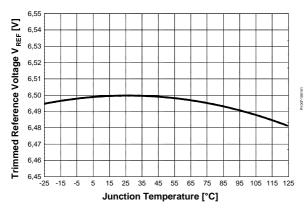
Figure 29 Trimmed Reference  $V_{REF}$  vs.  $T_i$
