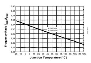
Figure 35 Frequency Ratio  $f_{OSC3}/f_{OSC4}$  vs.  $T_j$
