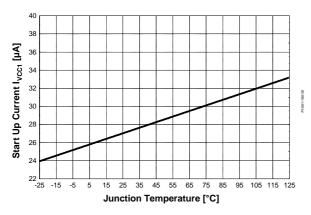
Figure 23 Start Up Current  $I_{VCC1}$  vs.  $T_i$
