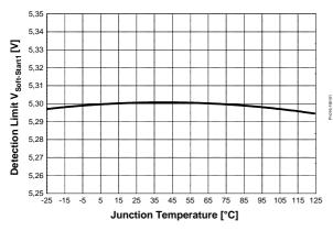
Figure 41 Detection Limit V<sub>Soft-Start1</sub> vs. T<sub>i</sub>
