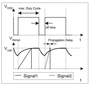
Figure 15 Dynamic Voltage Threshold V<sub>csth</sub>
