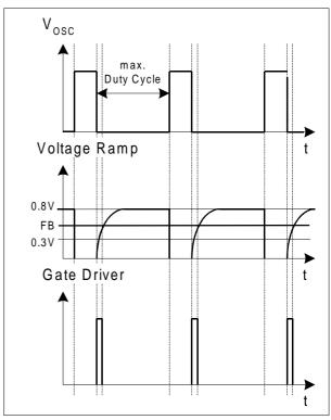
Figure 7 Light Load Conditions
