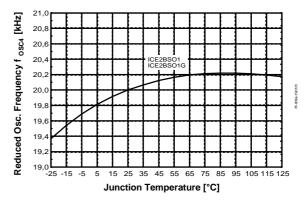
Figure 33 Reduced Osc. Frequency  $f_{OSC4}$  vs.  $T_i$
