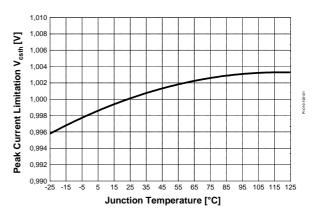
Figure 44 Peak Current Limitation  $V_{csth}$  vs.  $T_i$
