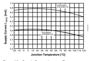
Figure 25 Supply Current  $I_{VCC3}$  vs.  $T_i$
