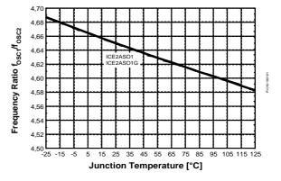
Figure 34 Frequency Ratio  $f_{OSC1}/f_{OSC2}$  vs.  $T_i$
