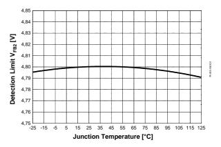
Figure 40 Detection Limit  $V_{FB2}$  vs.  $T_i$
