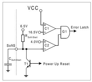
Figure 22 Overvoltage Detection
