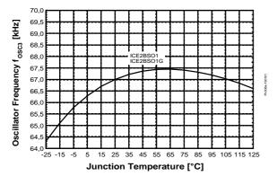
Figure 31 Oscillator Frequency  $f_{OSC3}$  vs.  $T_i$
