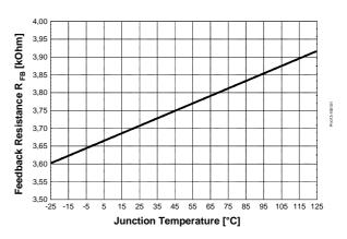
Figure 38 Feedback Resistance  $R_{FB}$  vs.  $T_j$
