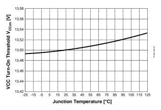
Figure 26 VCC Turn-On Threshold  $V_{VCCon}$  vs.  $T_i$
