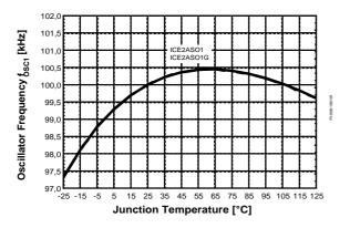
Figure 30 Oscillator Frequency f<sub>OSC1</sub> vs. T<sub>i</sub>
