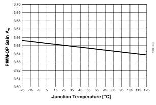
Figure 37 PWM-OP Gain  $A_V$  vs.  $T_i$
