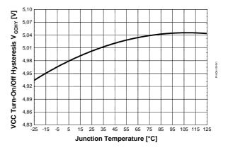
Figure 28 VCC Turn-On/Off Hysteresis V<sub>VCCHY</sub> vs. T<sub>i</sub>
