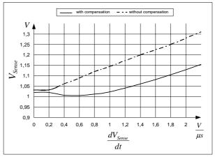
Figure 16 Overcurrent Shutdown
