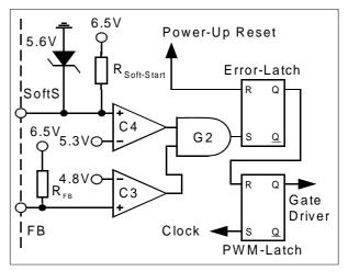
Figure 10 Activation of Protection Unit
