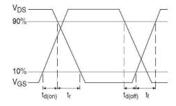
Fig 18b. Switching Time Waveforms
