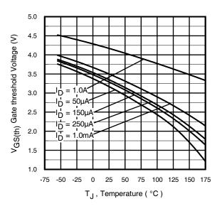
Fig 14. Threshold Voltage Vs. Temperature
