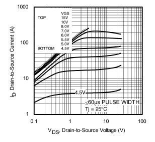
Fig. 1 Typical Output Characteristics
