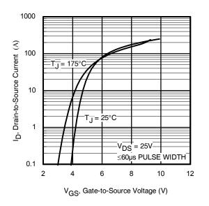
Fig. 3 Typical Transfer Characteristics
