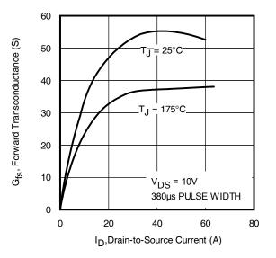
Fig. 4 Typical Forward Trans conductance Vs. Drain Current
