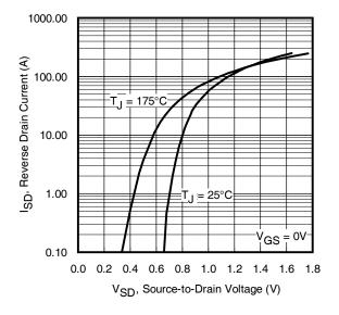
Fig. 7 Typical Source-to-Drain Diode Forward Voltage
