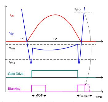
Figure 8: Resonant half-bridge operation waveform
