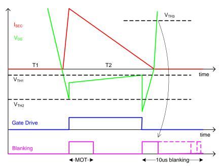
Figure 6: Secondary side DCM/CrCM operation
