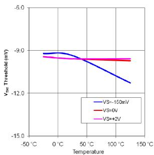
Figure 20: V<sub>TH1</sub> vs. Temperature and Common Mode (OVT=Floating)
