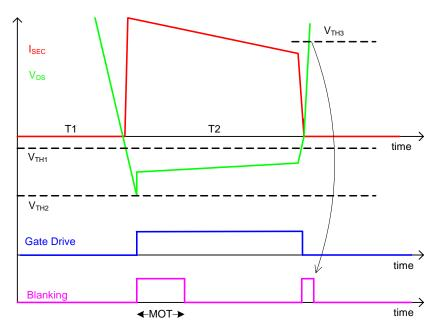
Figure 5: Secondary side CCM operation
