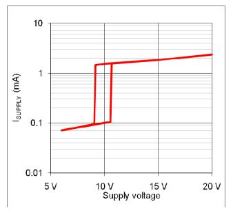
Figure 13: Supply Current vs. Supply Voltage
