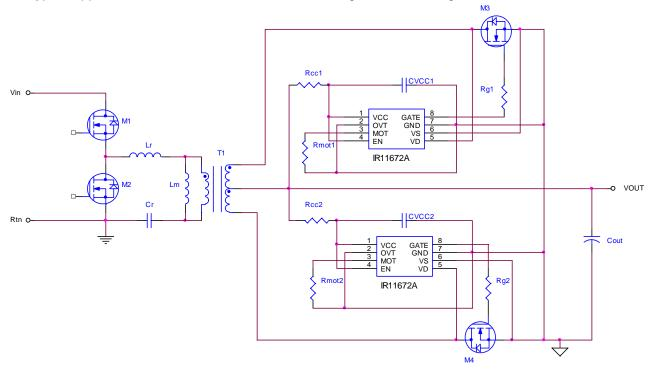
Figure 7: Resonant half-bridge application circuit
