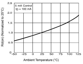
Figure 4. Typical Normalized On-Resistance
