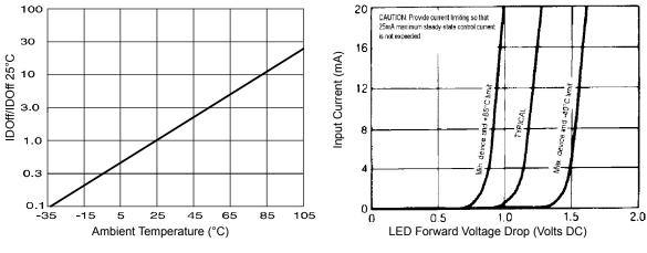
Figure 5. Typical Normalized Off-State Leakage
