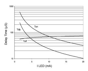
Figure 7. Typical Delay Times
