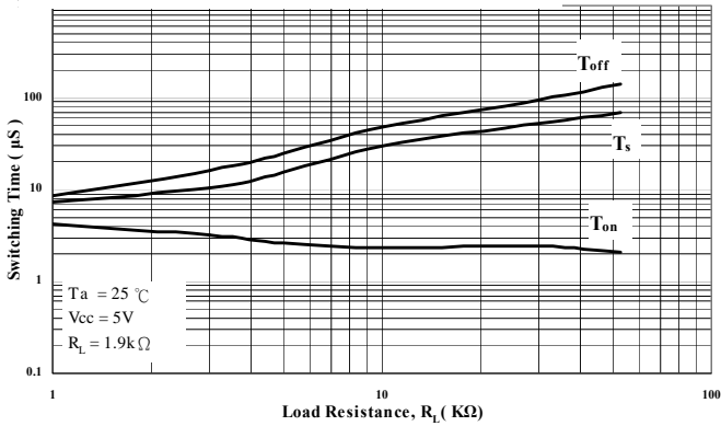
Figure 15. Switching Time vs. Load Resistance
