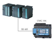
Example PLC communication with Profibus or Modbus
