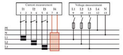
Figure: Connection for measurement channels and differential current transformer of series KBU (split core).
