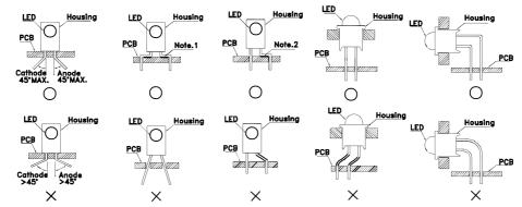
$^{\prime}\bigcirc$  " Correct mounting method "imes" Incorrect mounting method
