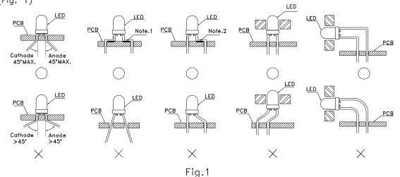
" $\bigcirc$ " Correct mounting method " $\times$ " Incorrect mounting method Note 1-2 : Do not route PCB trace in the contact area between the leadframe and the PCB to prevent short-circuits.
