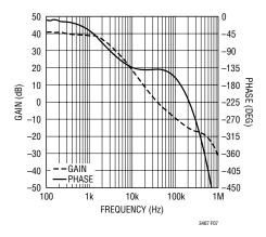
Figure 7.Bode Plot of 3.3V to 5V Application
