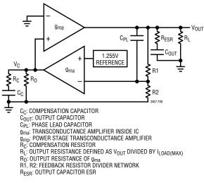
Figure 6. Boost Converter Equivalent Model
