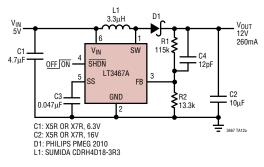
Figure 9. 5V to 12V, 260mA Step-Up Converter
