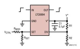
Figure 10. Voltage-Controlled Delay
