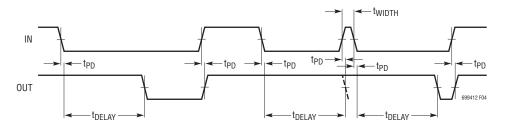
Figure 4. Falling-Edge Delayed Timing Diagram (LTC6994-1, POL = 1)
