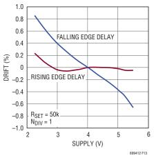
Figure 13. Delay Drift vs Supply Voltage
