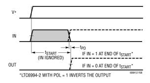
Figure 8. Start-Up Timing Diagram
