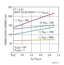
Figure 14. I<sub>S(ACTIVE)</sub> vs Input Frequency, LTC6994-1
