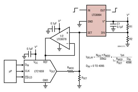
Figure 11. Digitally Controlled Delay
