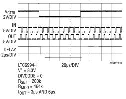
Figure 12. Typical Settling Time
