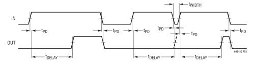
Figure 3. Rising-Edge Delayed Timing Diagram (LTC6994-1, POL = 0)
