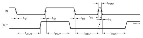
Figure 6. Both Edges Delayed (Inverting) Timing Diagram (LTC6994-2, POL = 1)
