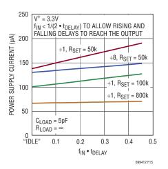
Figure 15. I<sub>S(ACTIVE)</sub> vs Input Frequency, LTC6994-2
