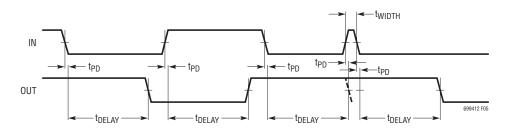
Figure 5. Both Edges Delayed Timing Diagram (LTC6994-2, POL = 0)
