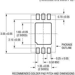
DCB Package 6-Lead Plastic DFN (2mm × 3mm) (Reference LTC DWG # 05-08-1715 Rev A)
