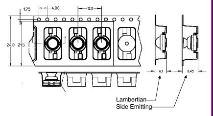
Figure 8. Reel dimensions and orientation.
