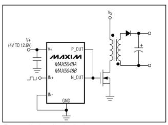
Figure 3. Noninverting Application
