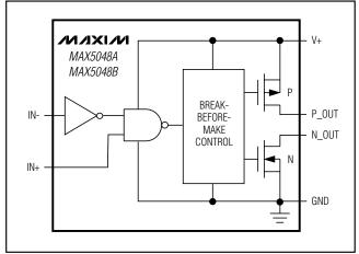
Figure 2. MAX5048A/MAX5048B Functional Diagram
