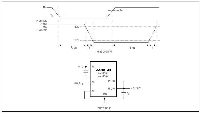
Figure 1. Timing Diagram and Test Circuit
