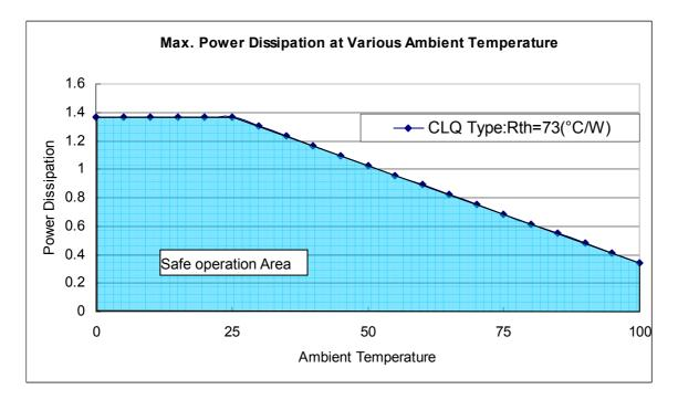
The maximum allowable package power dissipation is determined as  $P_D(max) = (Tj - Ta) / R_{th(j-a)}$ . When 24 output channels are turned on simultaneously, the actual package power dissipation is  $P_D(act) = (I_{DD} \times V_{DD}) + (I_{OUT} \times Duty \times V_{DS} \times 24)$ . Therefore, to keep  $P_D(act) \le P_D(max)$ , the allowable maximum output current as a function of duty cycle is:
