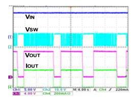
Fig. 84. Thermal protection
