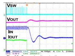
Fig. 82. Open-circuit protection
