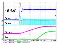
Fig 73. C<sub>IN</sub>=C<sub>OUT</sub>=Ceramic capacitor (2 x 4.7uF/35V)
