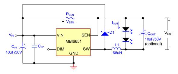
$C_{\text{IN}}\!\!:$  VISHAY, 293D106X9050D2TE3, D case Tantalum Capacitor  $C_{\text{OUT}}\!\!:$  VISHAY, 293D106X9050D2TE3, D case Tantalum Capacitor  $C_{\text{BP}}\!\!:$  TAIYO YUDEN, UMK212B7104MG-T, 0805 Ceramic Capacitor
