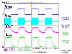
Fig 67. Dimming waveform  $(V_{IN}=12V, R_{SEN}=0.27, 2-LED)$
