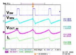
Fig 68. Switching waveform (12 $V_{IN}$ , 3.6 $V_{OUT}$ ,  $R_{SEN}$ =0.27 )
