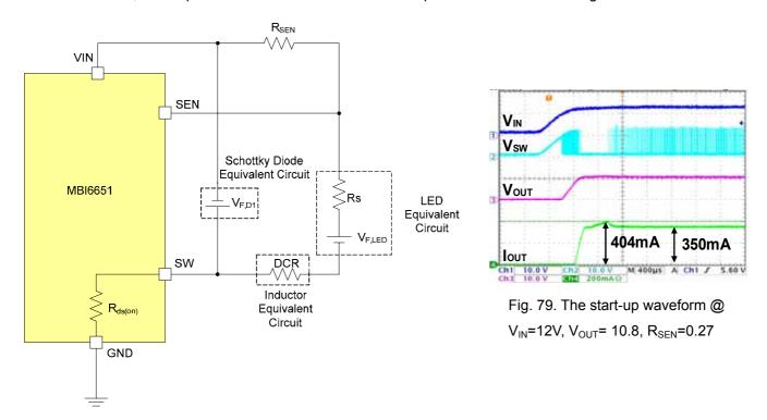
Fig. 78. The equivalent impedance in a MBI6651 application circuit
