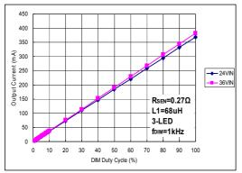
Fig. 80. DIM duty cycle: 1% ~ 100%
