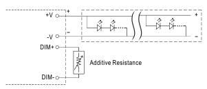
"DO NOT connect "DIM- to -V"
