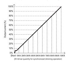
Dimming input: Additive resistance Note: 1. Min. dimming level is about 6% and the output current is not defined when 0%< Iout<6% 2. The output current could drop down to 0% when dimming input is about 0kΩ or 0Vdc, or 10V PWM signal with 0% duty cycle.
