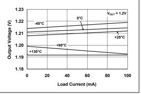
**FIGURE 2-10:** Output Voltage vs. Load Current.
