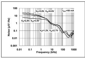
FIGURE 2-27: Output Noise vs. Frequency.
