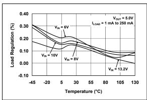
FIGURE 2-21: Load Regulation vs. Temperature.
