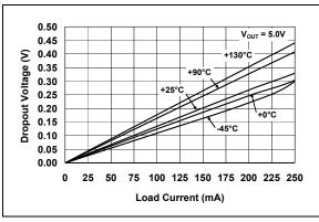
**FIGURE 2-15:** Dropout Voltage vs. Load Current.
