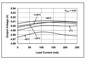
FIGURE 2-12: Output Voltage vs. Load Current.
