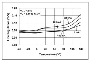
FIGURE 2-23: Line Regulation vs. Temperature.
