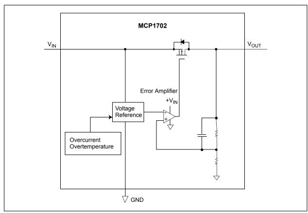
FIGURE 4-1: Block Diagram.
