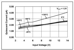
**FIGURE 2-1:** Quiescent Current vs. Input Voltage.
