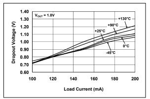
**FIGURE 2-13:** Dropout Voltage vs. Load Current.
