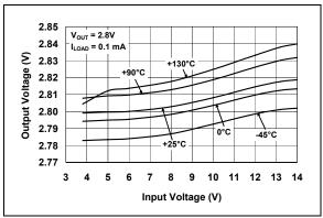
**FIGURE 2-8:** Output Voltage vs. Input Voltage.
