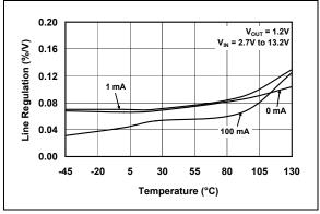
**FIGURE 2-22:** Line Regulation vs. Temperature.
