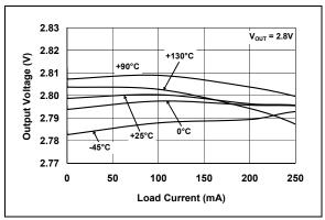
FIGURE 2-11: Output Voltage vs. Load Current.
