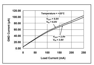
FIGURE 2-5: Ground Current vs. Load Current.
