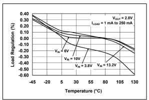
**FIGURE 2-20:** Load Regulation vs. Temperature.
