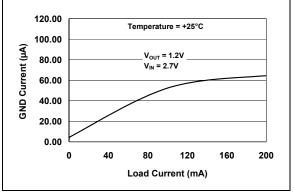
FIGURE 2-4: Ground Current vs. Load Current.
