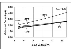
FIGURE 2-2: Quiescent Current vs.Input Voltage.
