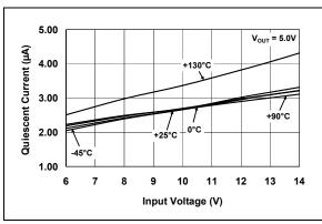
**FIGURE 2-3:** Quiescent Current vs.Input Voltage.
