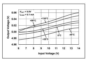
**FIGURE 2-9:** Output Voltage vs. Input Voltage.
