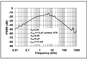
**FIGURE 2-26:** Power Supply Ripple Rejection vs. Frequency.
