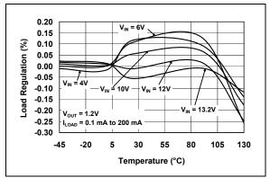
FIGURE 2-19: Load Regulation vs. Temperature.
