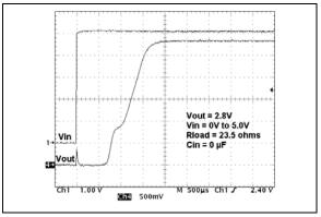
FIGURE 2-28: Power Up Timing.
