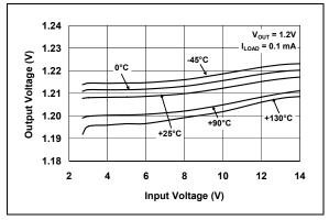
**FIGURE 2-7:** Output Voltage vs. Input Voltage.
