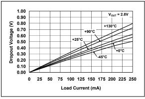
**FIGURE 2-14:** Dropout Voltage vs. Load Current.
