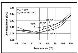
FIGURE 2-24: Line Regulation vs. Temperature.
