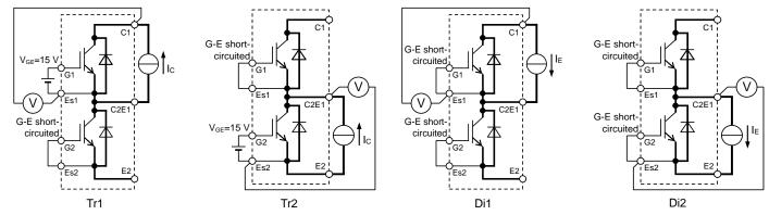
V<sub>CEsat</sub> characteristics test circuit
