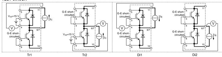
V<sub>CEsat</sub> characteristics test circuit
