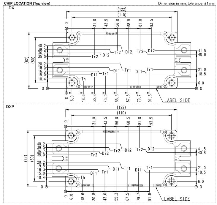
Tr1/Tr2: IGBT, Di1/Di2: FWD, Th: NTC thermistor
