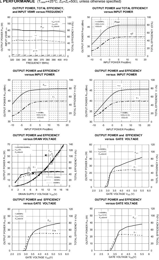
RoHS Compliance, 330-400MHz 30W 12.5V, 3 Stage Amp. For MOBILE RADIO
