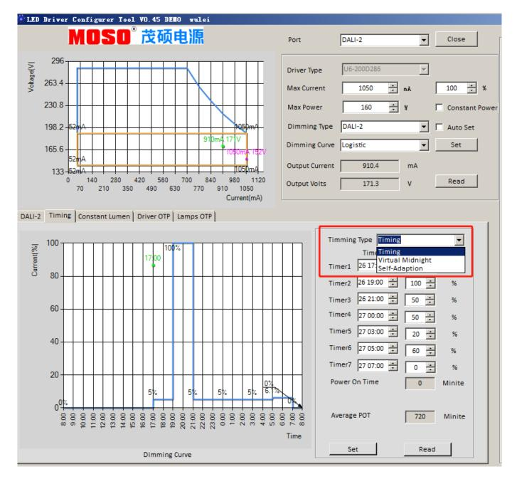
After selecting "Timing dimming", you can set the parameters related to timing dimming. The software supports three timing dimming settings: traditional timing, virtual midnight timing dimming, and adaptive timing dimming.
