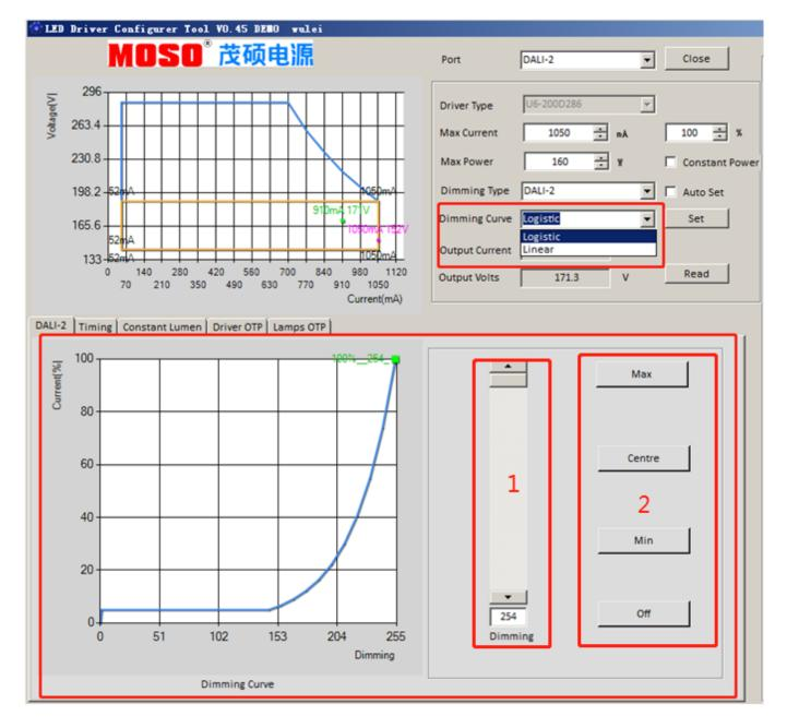
There are two types of dimming curves, logistic and linear. The figure is logistic. You can click the button in the red box 2 above to adjust the current coarsely, or click the button in the red box 1 to fine-tune the current.
