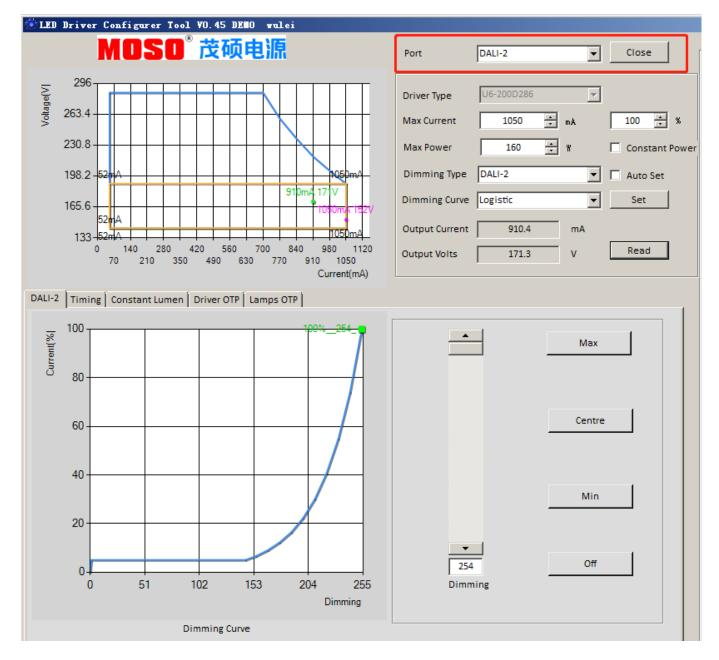
When the driver is turned on, one end of the DALI programmer recorder USB is connected to the computer, and the other end is connected to the driver dimming line.
