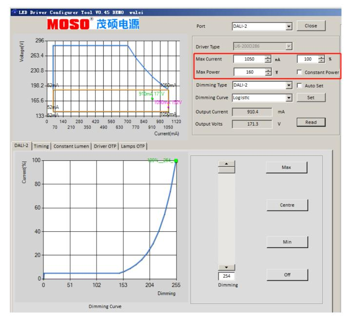
Set the output current of the LED driver and the maximum output power to ensure that the driver does not exceed the set maximum power usage (reduce the output current).
