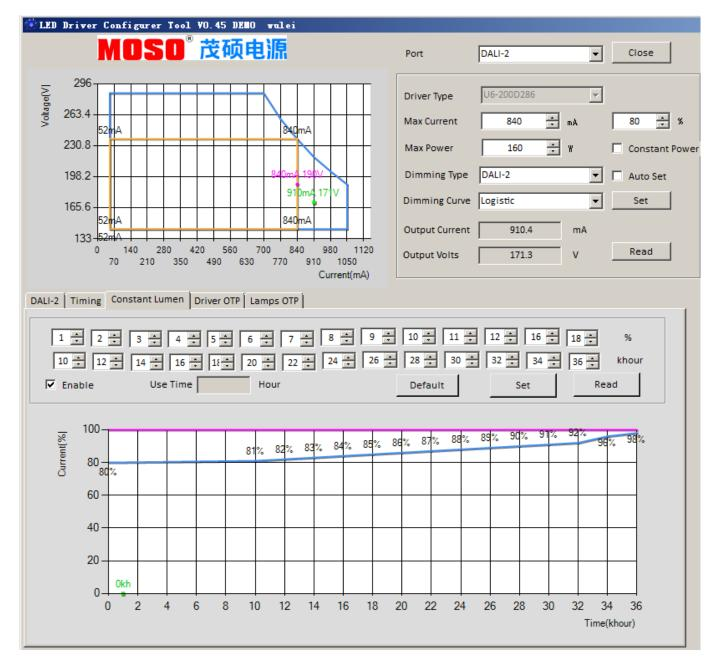
Select "Start CLO(Constant Lumen Output)", configure the working time and the corresponding compensation current percentage.
