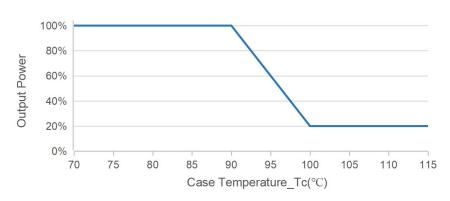
Notes: Customers can set the start derating temperature and end derating temperature. This curve is the default factory protection curve, When the temperature rises to the normal operating temperature, the drive will resume output.
