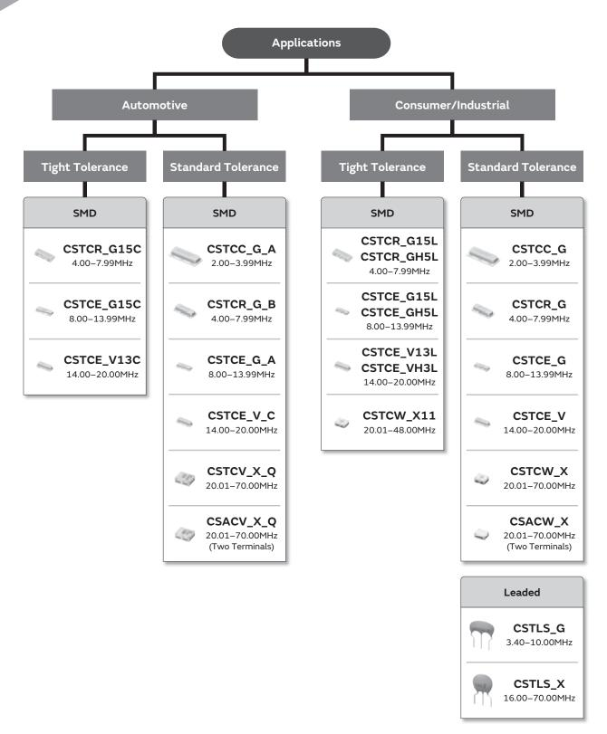
Notice: "CERALOCK® for consumer" and "CERALOCK® for automotive" is different in the specification of Operating Temperature Range, Environmental Characteristics, Physical Characteristics and so on. Please choose either "for consumer" or "for automotive" according to the required specification.
