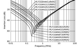
Common Mode Insertion Loss-Frequency Characteristics
