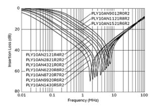
Differential Mode Insertion Loss-Frequency Characteristics
