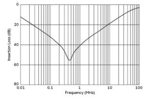
Common Mode Insertion Loss (Typ.)
