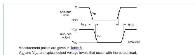
Input (nAn, nBn) to output (nBn, nAn) propagation delays
