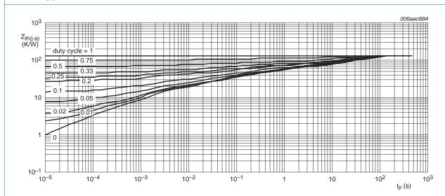
FR4 PCB, single-sided copper, mounting pad for collector 1 cm<sup>2</sup>
