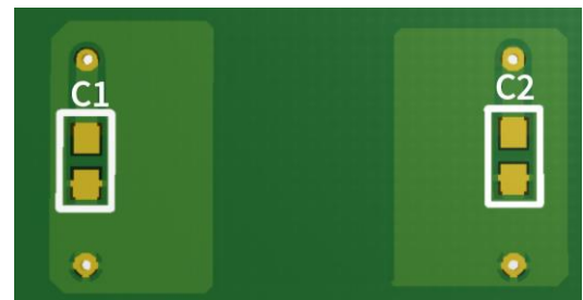
Figure8.3 Recommended PCB Layout — Bottom
