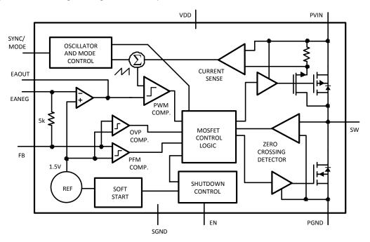
Figure 21. Simplified Functional Diagram
