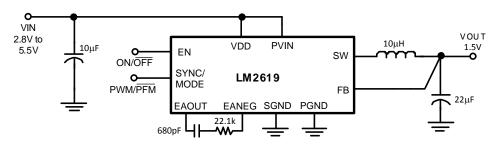
Figure 3. Typical Circuit for 1.5-V Output Voltage
