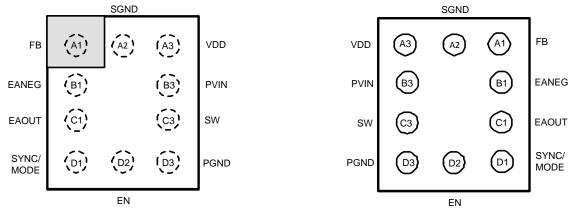
Figure 4. YPA Package Top View
