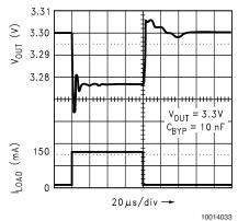
**Typical Performance Characteristics** Unless otherwise specified:  $C_{IN} = 1\mu$ F,  $C_{OUT} = 4.7\mu$ F,  $V_{IN} = V_{OUT}(NOM) + 1$ ,  $T_A = 25^{\circ}$ C, ON/OFF pin is tied to  $V_{IN}$ . (Continued)
